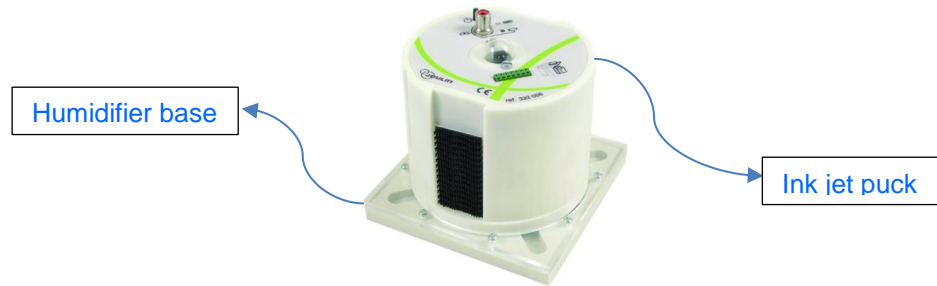
Puck on humidifier base.
