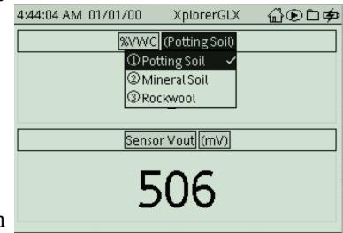
With the SPARK SLS, connect the Soil Moisture Sensor and select the soil type from the list of choices that will appear on the screen.
