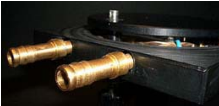
Fig. 7 Connection for cooling water circuit
